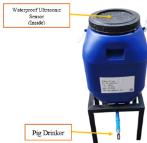
Figure 7 Water Tank of Project SwineTech
